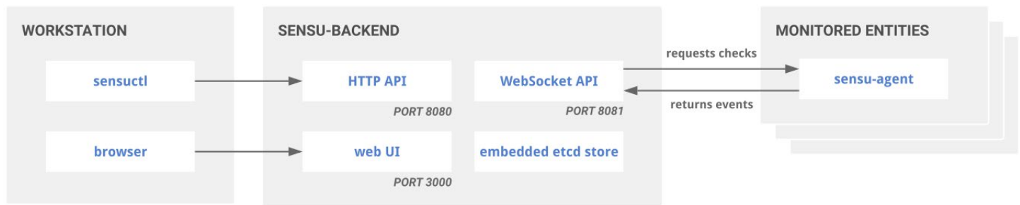
Sensu standalone architecture with embedded etcd
