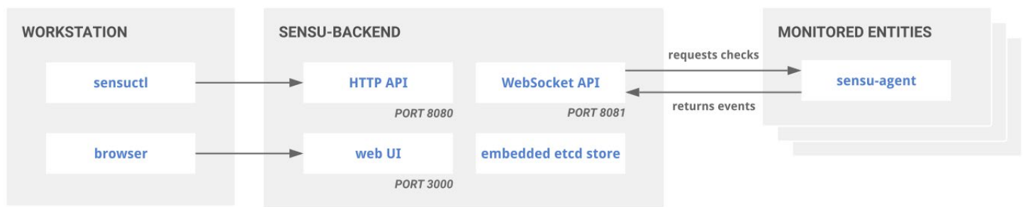
Sensu standalone architecture with embedded etcd
